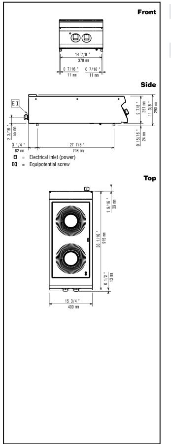
Supply voltage: 380-400 V/3N ph/50/60 Hz Predisposed for: 380-400V 3N~ 50/60Hz 6-6,8kW **Total Watts:** 6.8 kW **Key Information:**
